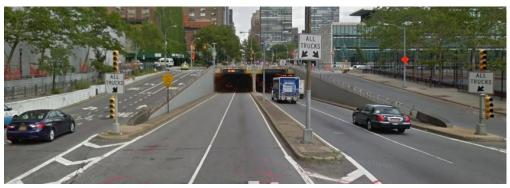
Figure 35. Example of a confusing truck route signage.
