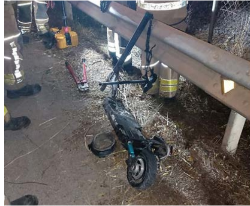
Figure 4. State of the PMV on fire. Source: FGC.
